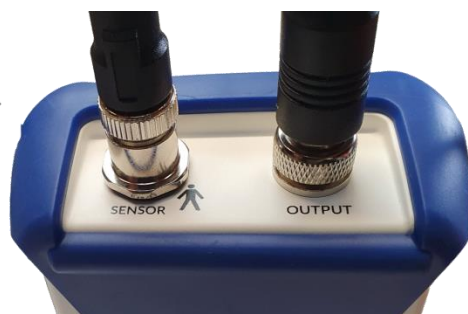
Tighten cable connectors fully
